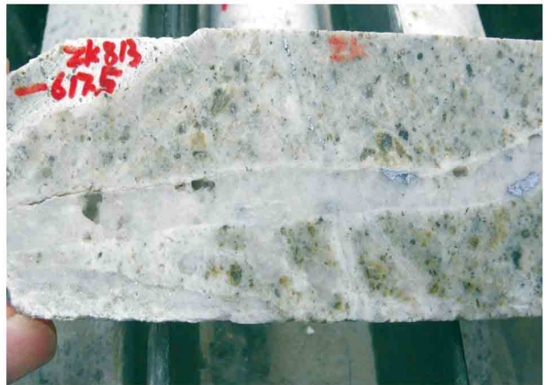
图1 甲玛矿区 ZK813 钻孔中斑岩的矽卡岩化现象 Fig. 1 Skarnization in porphyry from ZK813 drill hole
